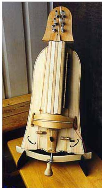
More than 300 hours of work goes into the making of one of these instruments. Special tools and jigs are constructed, formers made and woods specially selected for the wide variety of uses the hurdy-gurdy demands to achieve the best possible acoustic and playing qualities.
